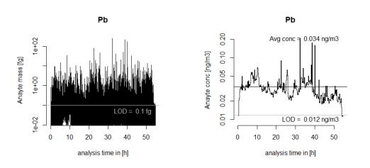
Pb content in industrial indoor air. Signal measured in 1 s intervals over 50 h (left). The same signal averaged to 10 min intervals and considering the actual volume flow (right).
