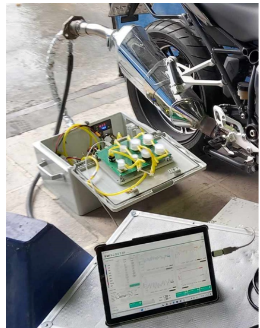
Fig. 1: Experimental setup for motorbike measurements
